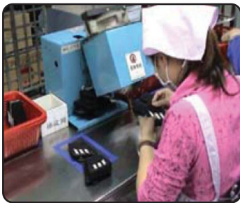
Glue on upper in line, laminates the upper and the hook & loop 用於拖鞋鞋面黏黏扣帶
