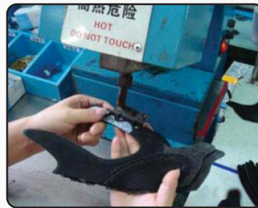
Glue on upper in line, laminates the upper and the hook & loop 用於拖鞋鞋面黏黏扣帶
