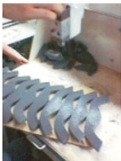
Glue on upper in line, laminate the upper and the hook & loop 用於拖鞋鞋面黏黏扣帶
