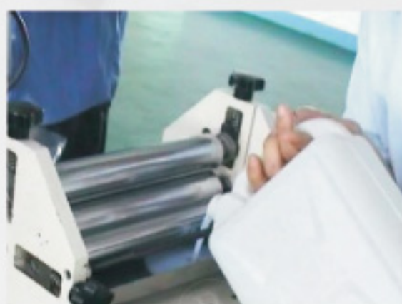
Pour in water based cement
